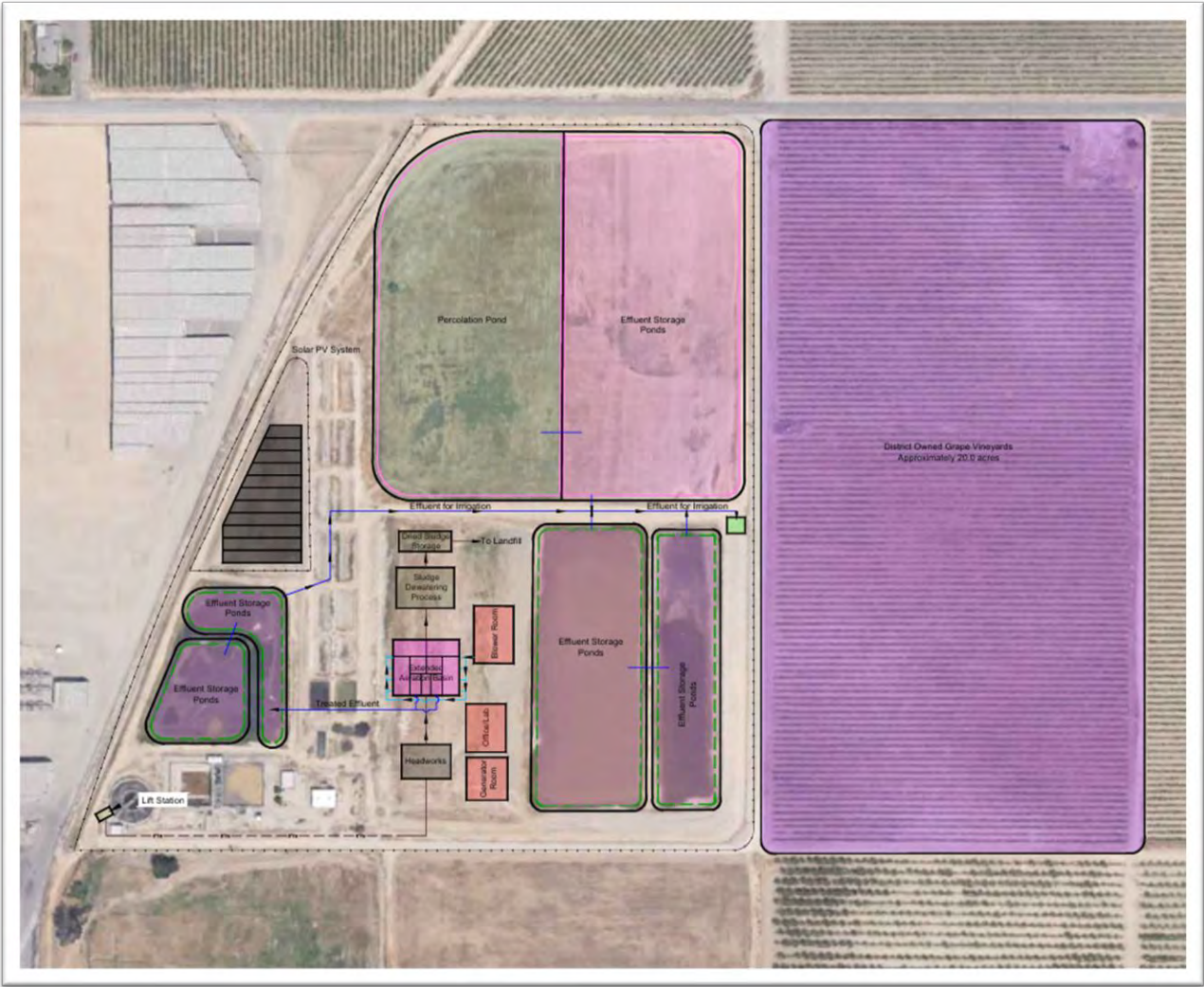
Figure 3 – Project Site Map Proposed WWTP Improvement Layout
